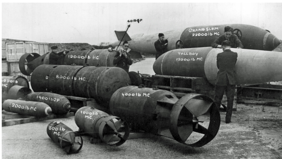
Photo 19: British bombs. At the top is the massive ‘Grand Slam’, weighing 11 tons and allegedly capable of penetrating 7 m+ of reinforced concrete.
