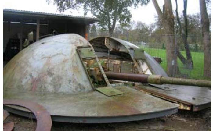
German Flak (AA) gun, S.K.C. 32, 105 mm with copula. Guns were installed in Regelbau Fl 243 bunkers with compartment for a crew of 15. Awaiting restoration at museum in Aalborg.
