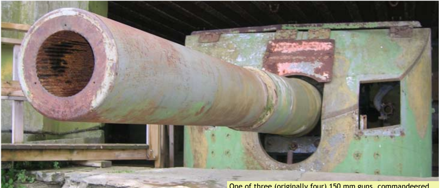
One of three (originally four) 150 mm guns, commandeered from the Danish coastal defense ship "Niels Juel". German design (Krupp) and Swedish manufacture (Bofors).
