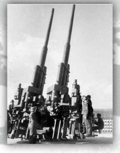
weapon, especially used on the Flak Towers. Capable of throwing a 26 kg shell almost 21 kilometers and with a maximum altitude of nearly 15 kilometers with a cadence of 20 rounds per minute, this was a formidable and respected adversary for the Allied airmen.
